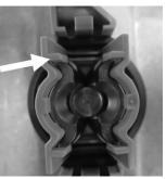
**8** Check if the clamps are attached correctly.
