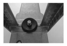
Position the coupler support on the actuator spindle, with the indicators facing you.
