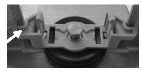
Position the clamps on the spindle head. Position the clamp parts to the groove of the spindle and in the small slot of the coupler support. They should not slip around.
