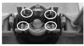
**9** Snap the clamp holder down to the coupler support.
